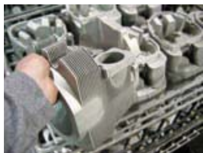
Fig. 2. Load of aluminum castings for heat treatment at a commercial shop (Photograph courtesy of Wisconsin Oven Corporation; East Troy, Wis.)
