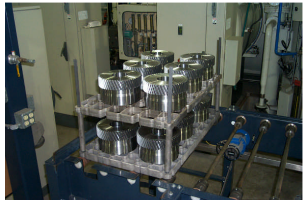
Figure 2: Load of Production Gears (650 lbs net) in Position for Loading into a Vacuum Carburizing Furnace followed by High Gas Pressure or Oil Quenching
