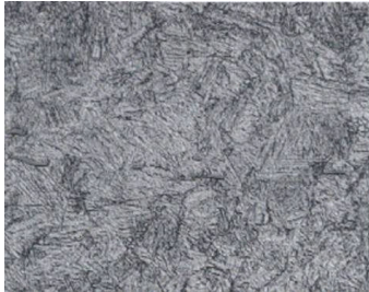
Atmosphere or Vacuum Carburized & Oil Quenched Sample. Core microstructure consists of tempered martensite. Core Hardness is 37 HRC.
