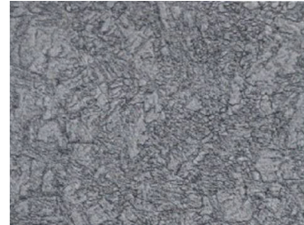
Vacuum Carburized & Gas Quenched Sample. Core microstructure consists of tempered martensite and transformation products. Core Hardness is 29 HRC.
