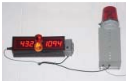
Fig 2 Plant-wide energy monitoring device [4]. The number on the left is the KW that the shop is currently running at. The number on the right is the peak already attained for the month. As you approach the peak, alarms are sounded. Ramping rates can immediately be cut back (or put on hold if possible) and auxiliary items (blowers, etc.) can be turned off. Cost of the monitor is about $3,000, and has a typical payback of 1 to 6 months.
