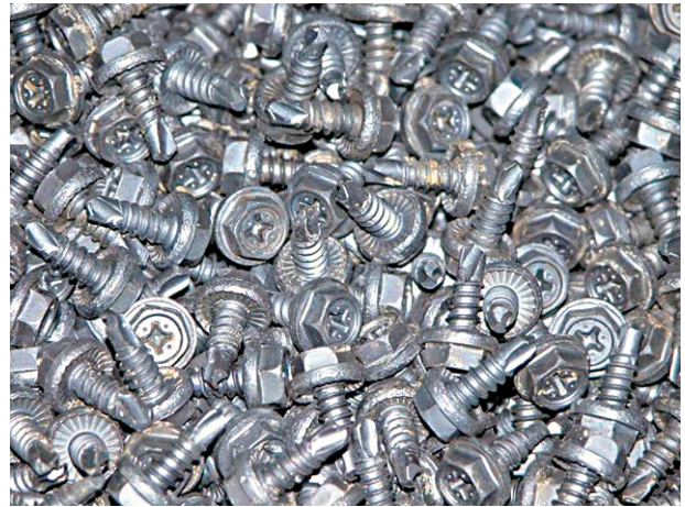
Fasteners should be cleaned prior to heat treatment.
