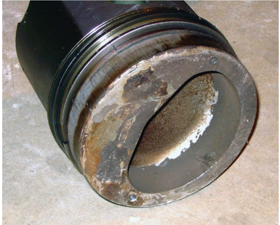
Fig. 2. Piston Head Component From Failed Power Generation Engine (photograph courtesy of Materials Engineering Inc.)
