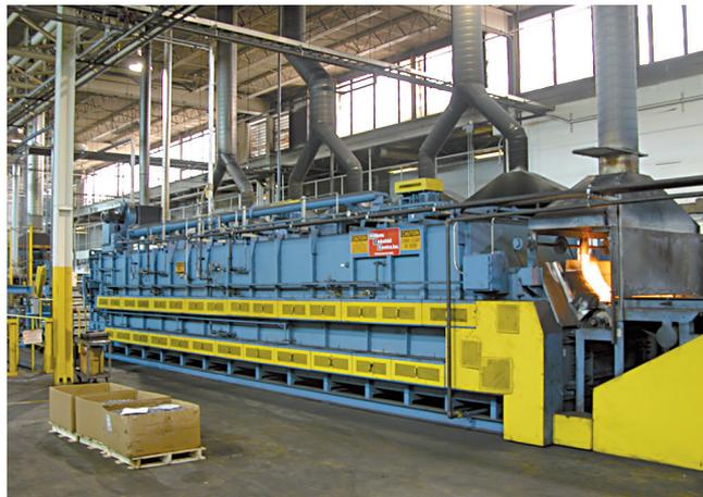
**Fig. 3 — Mesh belt conveyor furnace for hardening and case hardening fasteners (photograph courtesy of Williams Industrial Furnaces).**
