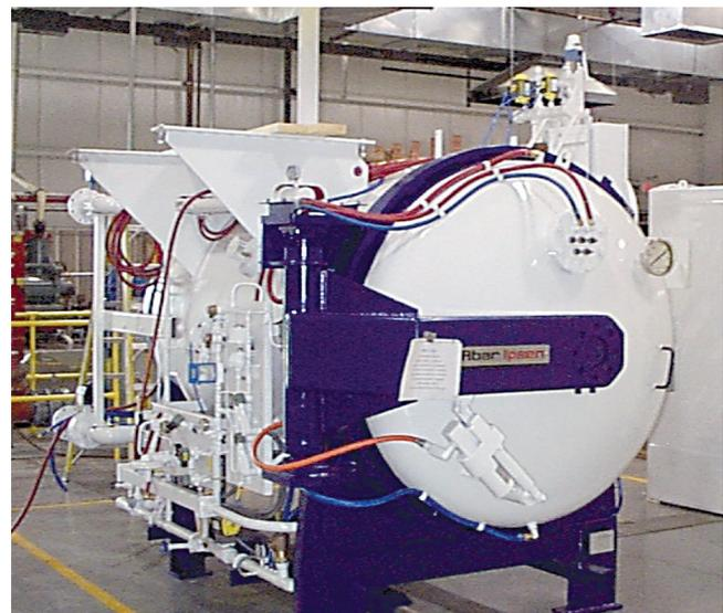
**Fig. 4 — Batch vacuum furnace (photograph courtesy of Ipsen USA).**
