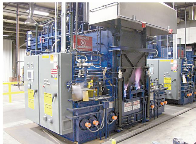
**Fig. 2** — Batch style integral quench furnace (photograph courtesy of Surface Combustion, Inc.).
