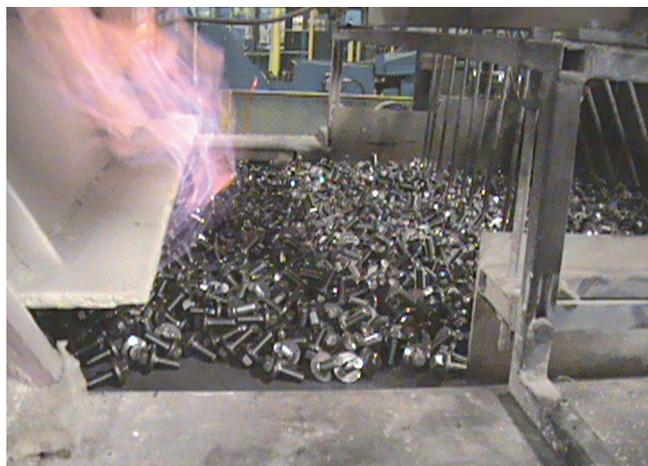
**Fig. 1** — Typical production load of fasteners entering a furnace for hardening.
