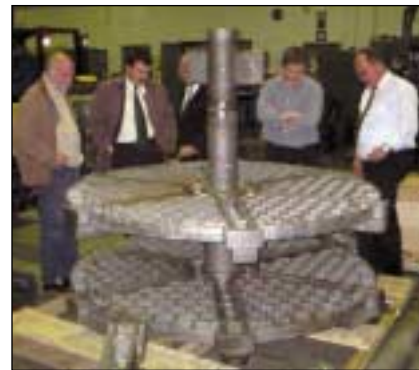
Fig. 3 — Pit furnace lifting post fixture. The fixture is being inspected by Michael Haite (right, in white shirt), director of alloy fabricator AFE Klefisch, Hürth, Germany, and engineers of customer Timken România S.A., Ploiesti. Photo courtesy North American Cronite Inc., Div. AFE Technologies Corp., North Ridgeville, Ohio.
