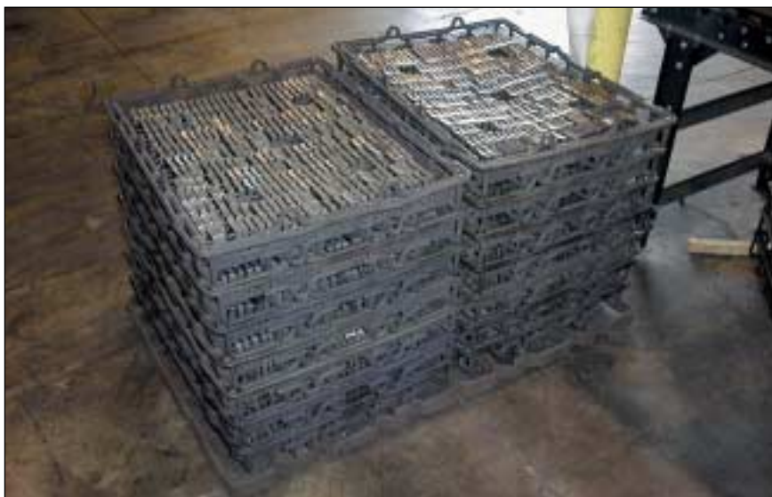
Fig. 1 — Baskets of precision-machined AISI/SAE 8620 (UNS G86200) steel plates will be carburized and oil quenched in a batch integral quench furnace. The parts baskets are made of AISI 330 (UNS N08330), an austenitic Ni-Cr-Fe-Si alloy combining resistance to carburization and oxidation at temperatures to 2200°F (1200°C) with high strength. Photo courtesy Specialty Heat Treating Inc., Grand Rapids, Mich. ( www.specialtyheat.com ).
