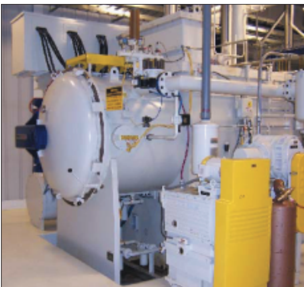
Fig. 2 — Carburizing chamber of the low-pressure carburizing furnace.
