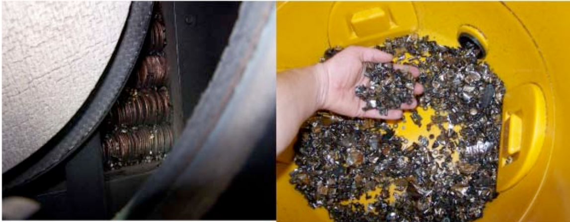
Figure 3 Small Parts Embedded in the Heat Exchanger System (Photograph Courtesy of SECO/WARWICK Corporation)
