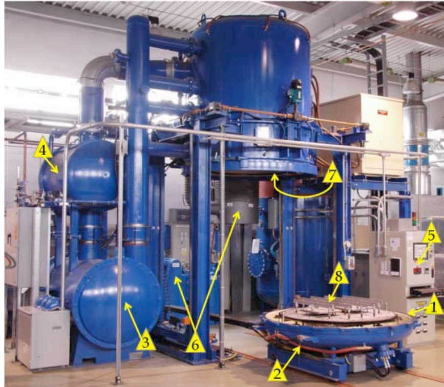
Figure 3 Typical Vertical Vacuum Furnace Maintenance Areas (Photograph Courtesy of Vac-Aero International)
