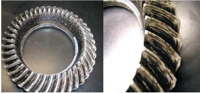
Fig. 1 — Unacceptable part surface appearance; parts after heat treating can include conditions such as blackened quench-oil stains, a coating of sludge, or scaly decarburized surfaces. Courtesy of D. Scott Mackenzie, Houghton International Inc., Valley Forge, Pa.
