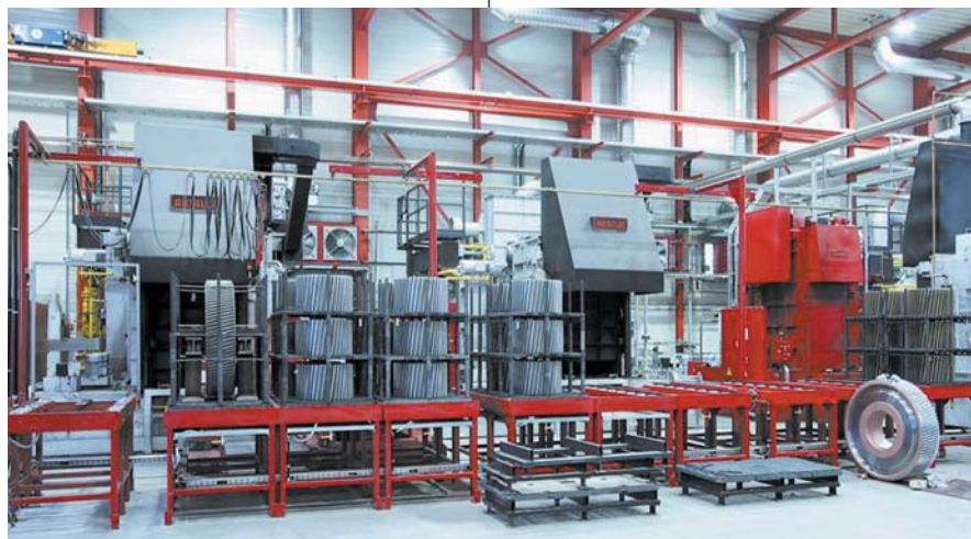
Wind-energy and mining gears for heat treatment in a batch IQ furnace. Courtesy of Aichelin Heat Treatment Systems, Plymouth, Mich.
