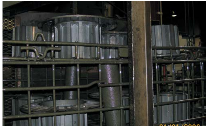
Fig. 2 — Acceptable part surface appearance; parts coming out of hardening and carburizing furnaces are clean, typically being gray-green in the as-quenched condition, with no evidence of loose soot, scale, or other contaminants on their surfaces. Courtesy of Specialty Heat Treating, Grand Rapids, Mich.
