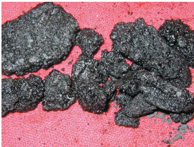
Fig. 4 - Fractionation of quench oil in the form of a carbonaceous residue.
