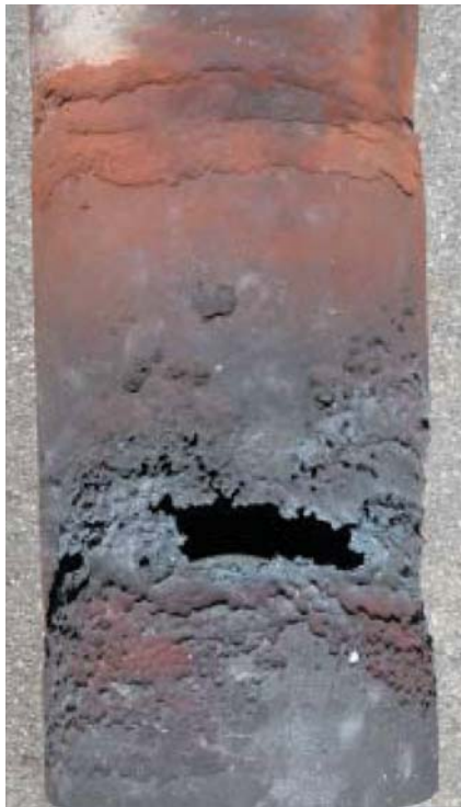
Fig. 1 — Top section of a radiant tube damaged by soot accumulation in the insulation.
