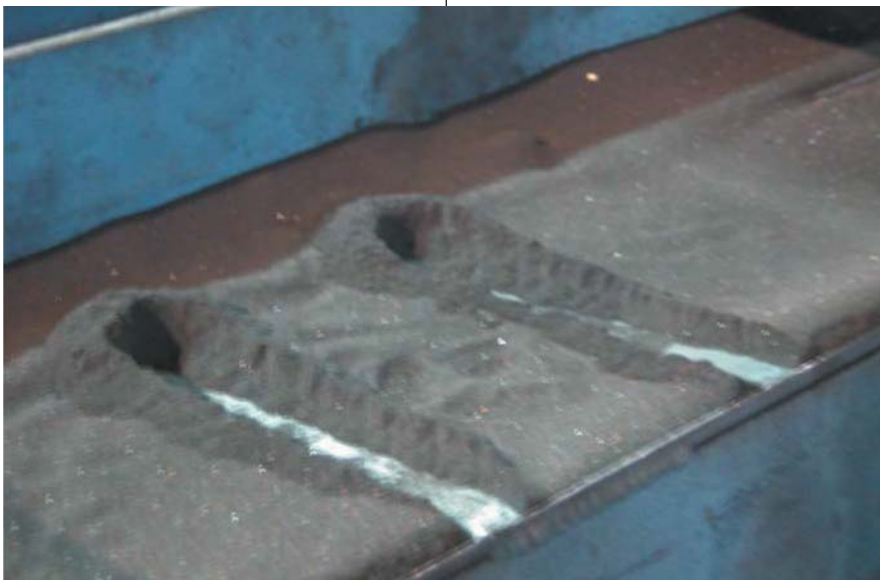
Fig. 2 — Soot formation on the front load table of a mesh-belt furnace after one hour with a furnace atmosphere out of control.
