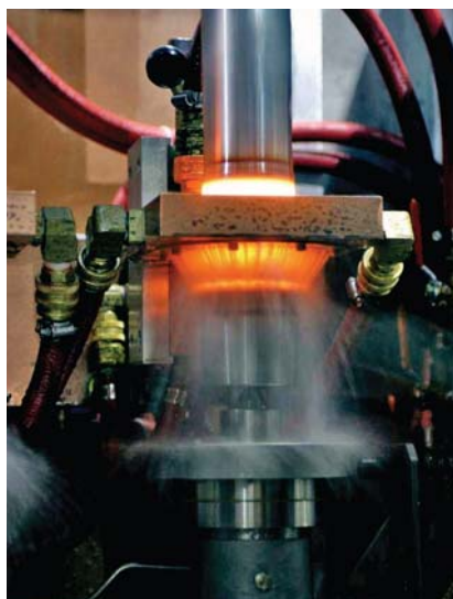
Fig. 2. Steering component heated with a machined single-turn coil
