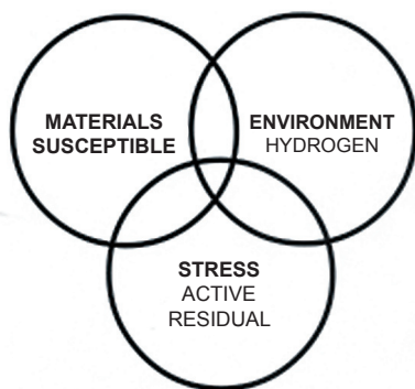
Fig. 1 — Factors contributing to stress corrosion cracking.
