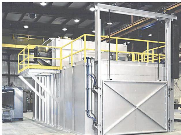
**Fig. 1 — Typical stress relief oven for wire coils (photo courtesy of Wisconsin Oven).**
