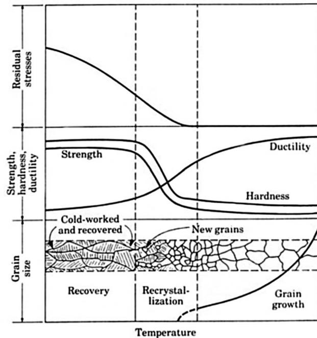
Fig. 2 — Effects of recovery and recrystallization on grain structure.
