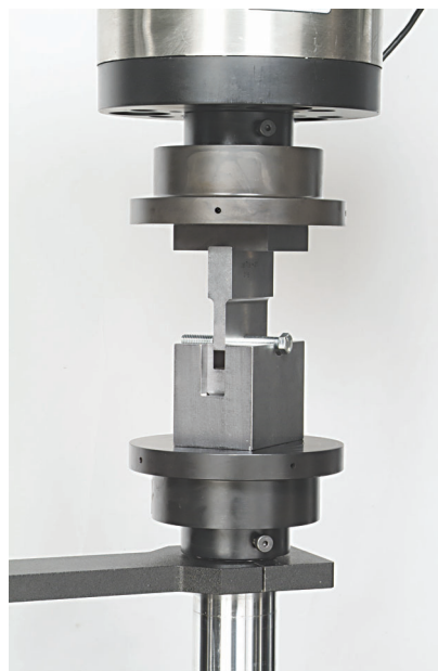
Fig. 4 — Double shear testing apparatus (photo courtesy of Instron®).
