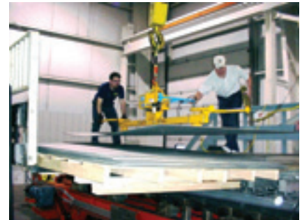
Fig. 3. Load of titanium sheet for vacuum age hardening (Photograph Courtesy of Solar Atmospheres of Western Pennsylvania)
