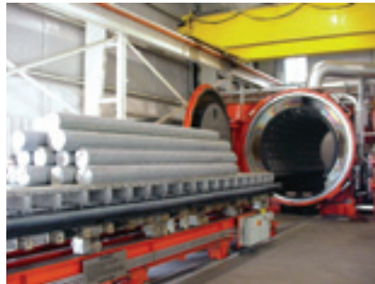
Fig. 2. Load of titanium ingots for vacuum degassing (Photograph Courtesy of Solar Atmospheres of Western Pennsylvania)
