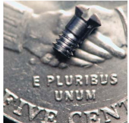
Fig. 8. Vacuum-carburized medical fastener (Photograph courtesy of Midwest Thermal-Vac)
