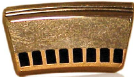
Fig. 1. Channel-wall braze joints (Photograph courtesy of GenCorp Aerojet)
