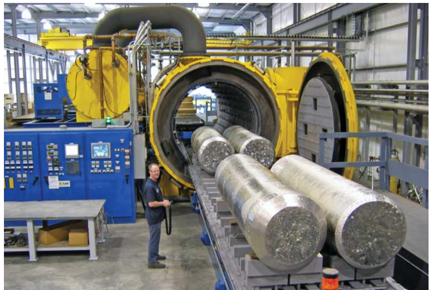
Fig. 9. Vacuum homogenizing of titanium ingots (Photograph courtesy of Solar Atmospheres)
