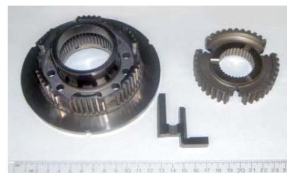
Fig. 6. Clutch and synchronizer hubs after LPC+HPGQ – SL-5506 material (Photograph courtesy of Stackpole Ltd.)
