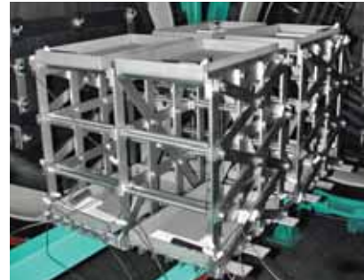
Fig. 4. TUS rack with metallic-sheathed thermocouples (Photograph courtesy of Vac Aero International Inc.)
