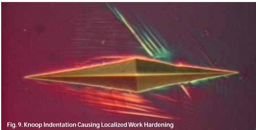
Fig. 9. Knoop Indentation Causing Localized Work Hardening
