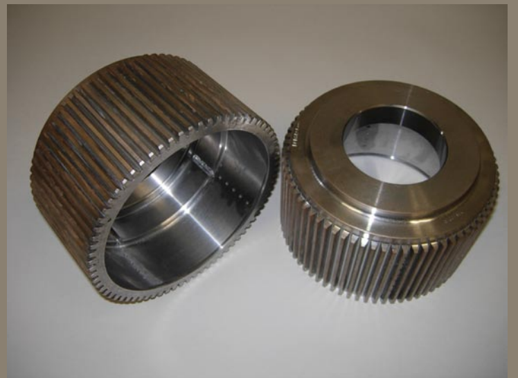
Figure 5: 6" Clutch Hub, Test Gear Type "C"
