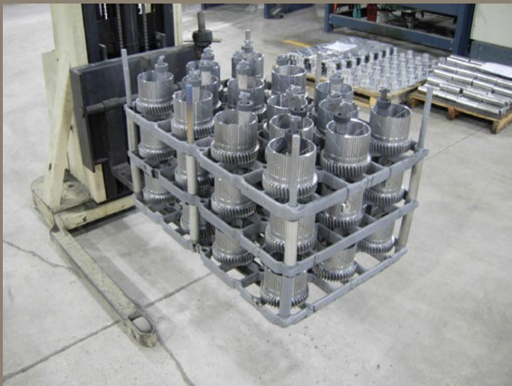
Figure 2: Typical Furnace Test Load (850 Pound Gross Load)
