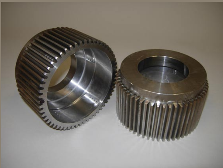
Figure 4: 4" Clutch Hub, Test Gear Type "B"
