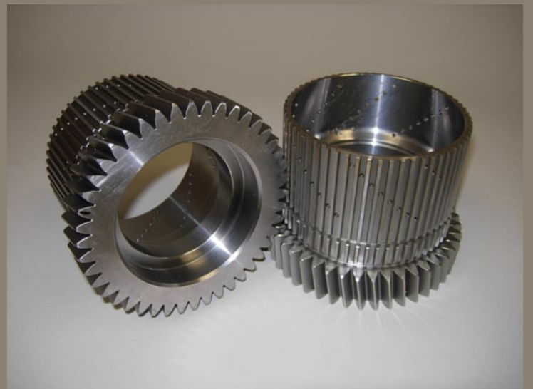
Figure 3: Clutch Gear, Test Gear Type "A"
