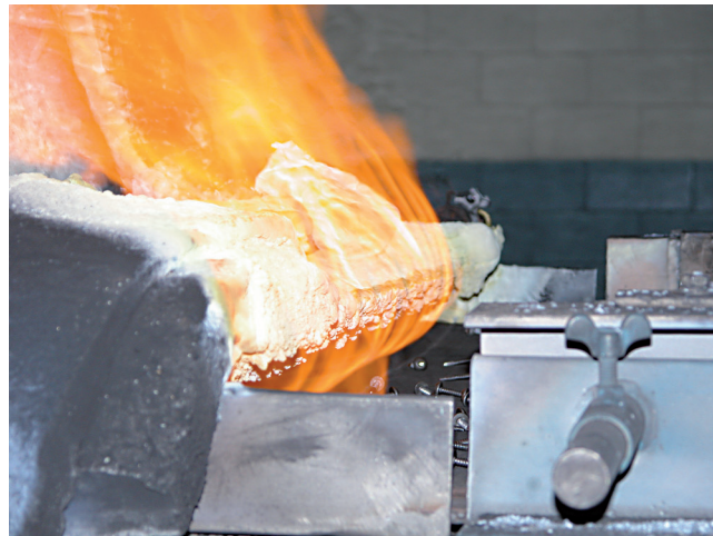
Fig. 2 — Residue buildup on the entrance end of a continuous mesh belt furnace due to wet/oily parts entering the system.
