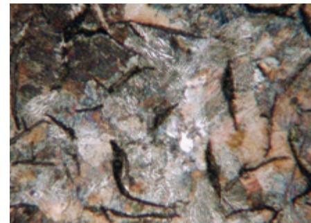
Fig. 3. Pearlitic structure of a cryogenically treated gray cast iron brake rotor; 100x; 2% nital etch. Courtesy of Controlled Thermal Processing Inc.
